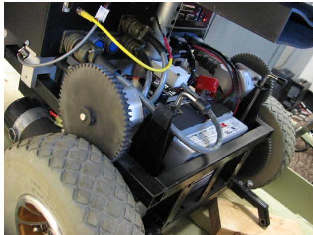
Electric powered wheelchair encoders built at HERL and used to record wheel speed and detect wheel slip in this study
