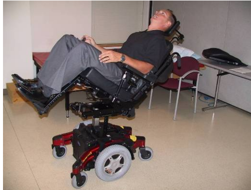
A power wheelchair with tilt-in-space, recline, and elevation functions
