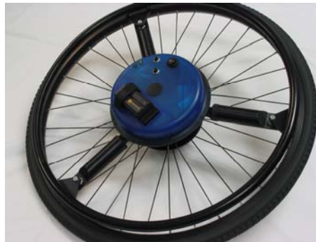
The SmartWheel, a device invented at HERL to collect wheelchair propulsion data
