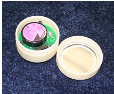
HERL researchers built dataloggers like the one pictured here to collect data manual wheelchair users' physical activity
