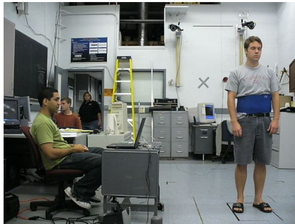
Tomás (L) records data from a sensor attached to the blue waist strap at the Human Movement and Balance Laboratory, while the cameras in the background record motion.
