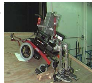
Power wheelchair being tested for static stability
