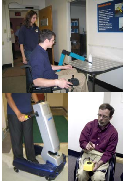
Three examples of HERL integrated control systems: the wheelchair mounted robotic arm (top), the robotic walker (left), and isometric joystick (right)
