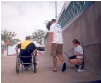
In this study, we measured the force needed to propel one's wheelchair across various surfaces, ramps, and to 'wheelie' for 10 feet
