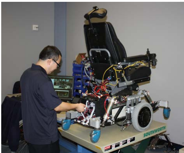
HERL postdoctoral student Hongwu Wang sets up the PerMMA Gen II prototype. Note the large center driving wheels and the blue caster wheels that lift the center wheels off the ground when climbing.
